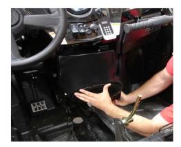
Once the enclosure is in, you will lift it into position, lining up the 2 holes on the front and the single hole on the side as indicated below
