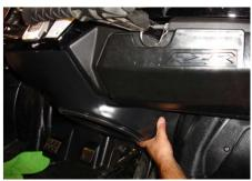
Using your left hand, apply upward pressure to the enslosure pressing it to the firewall and lining up the mouting nut to the hole in the firewall where the torx was removed
