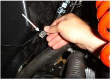
Remove the clip that held the screw fron the inner passenger wheel well, you will not use the clip and the torx that were removed
