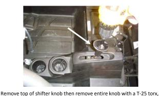
then remove all the T-25 torx around the center console and remove
