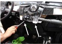
Locate the mounting holes on the front side of the enclosure, Using the screws provided, mount these screw through the metal bracket through the holes in the RZR dash
