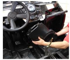
From the passenger side, slide/lift the enclosure into place, This will be slightly more difficult if you have power steering, you will need to go in at an angle and get the power steering provision around the power steering box
