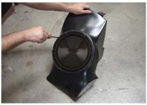
We recommend pre drilling the holes using a 1/8" drill bit to make screwing in the subwoofer easier. Connect the speaker inside to the speaker wire you ran into the enclosure and screw the speaker in tightly into the enclosure. NOTE: Sealing holes to prevent air leaking will improve sound quality. At this time, double check all the screws holding the mounting brackets on for tightness, make sure they are secure before installing
