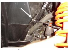
While holding the enclosure with your left hand, screw the provided screw into the mounting tab and nut with your right hand, be sure to line this up and begin to thread the screw with your hand to avoid stripping out the nut, once you can easily thread the screw into the nut and you are sure it is lined up, use a screwdriver to tighten the enclosure to the firewall
