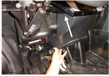
Locate the mounting hole on the driver side of the enclosure, Using the screw provided, mount this screw through the metal bracket through the hole in the RZR dash
