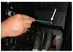
Remove the T-27 torx screw from the "firewall" directly above the floor opening where the lower panel and upper panels meet
